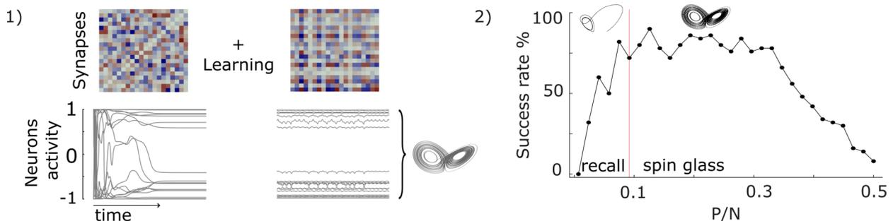
**Figure 1.** The Hopfield network has symmetric synapses and the neural activity relaxes to fixed point. **(1)** Learning introduces asymmetries that allows the network to autonomously reproduce the target dynamical system. **(2)** The success rate strongly depends on the number of patterns ( $P$ ) stored in the synaptic matrix before learning (The number of neurons is fixed at  $n = 10^3$ ).
